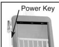
In order to limit battery consumption, the video display can be turned OFF by pushing the power key. Go to the settings menu to choose if the video screen will shut off after 5, 10, 15 or 20 seconds. If you do not want to use the Video off countdown, press "-" until you see "OFF" instead of numbers over the "-".
